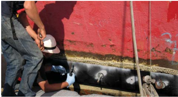
Independence Seaport Museum technicians applying a patch to the hull of the Olympia . Photo courtesy the Independence Seaport Museum.
